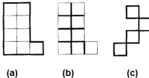
Figure 3: The perimeters and their relations: (a) the perimeter of an L-shape; (b) the contact perimeter of this same L-shape; (c) a shape without contact perimeter. Source: modified from [23].
