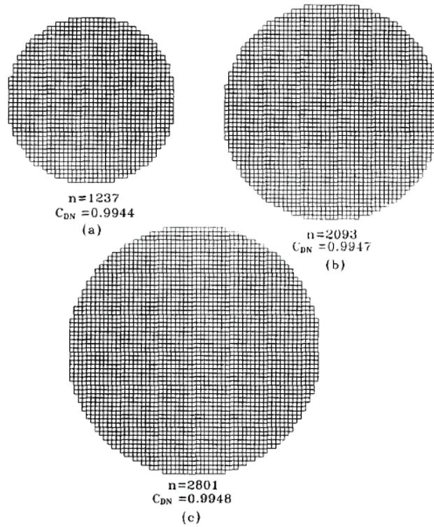
Figure 4: Examples of three different levels of resolution for a digital circle: (a) the digital circle composed of 1237 pixels; (b) the digital circle composed of 2093 pixels; (c) the digital circle composed of 2801 pixels; source [23].
